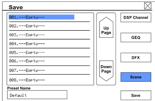
In order to access this page, press the "Save" button on the following pages: Channel, FX1-2 and System. You can save all settings to the internal memory of the GIG-202 Tab. You can save the DSP channels (48 presets), GEQ (48 presets), DFX (104 presets) and Scene (24 presets) which include all adjustments made in the mixer, including the ones mentioned above.
