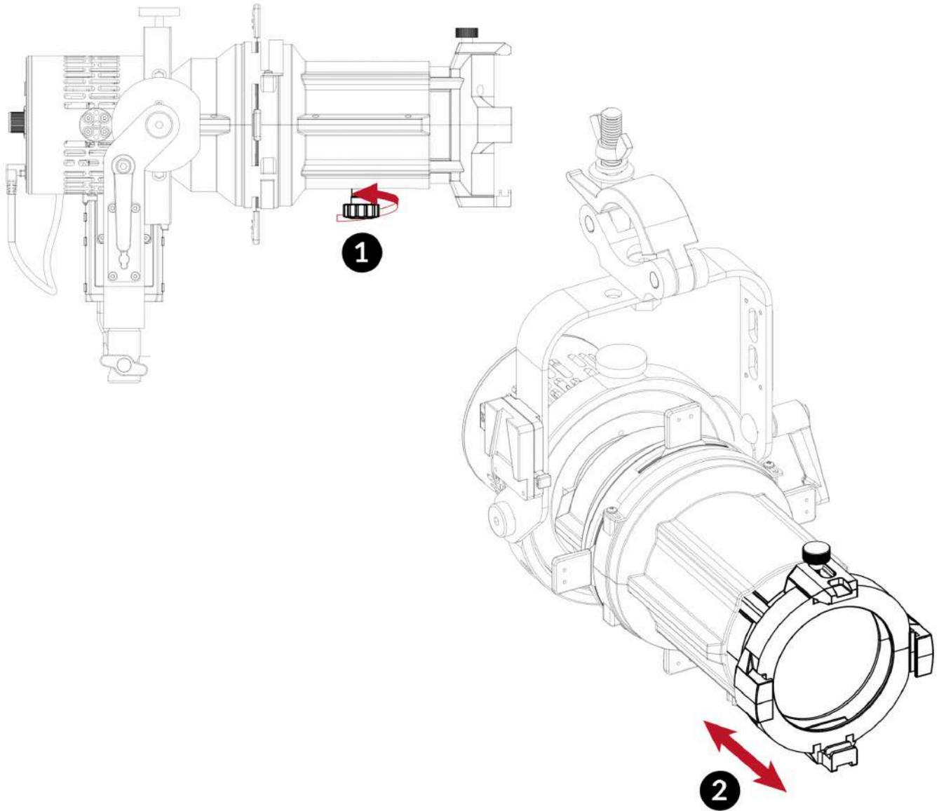
Turn the pin (1) and the lens tube will release, pull the lens tube outward allowing fully extended (2).
