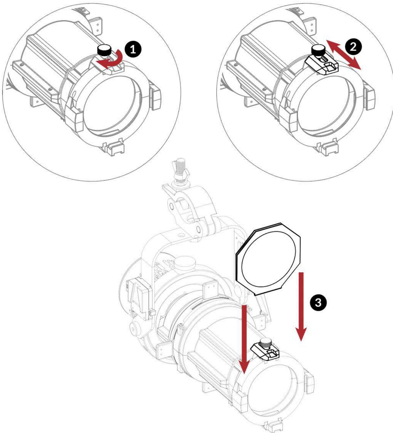
Rotate the pin (1) to release the cap. Push the cap in to create space for the Gel Frame holder (2) to slide in. Then, turn the pin (1) clockwise to secure it.
