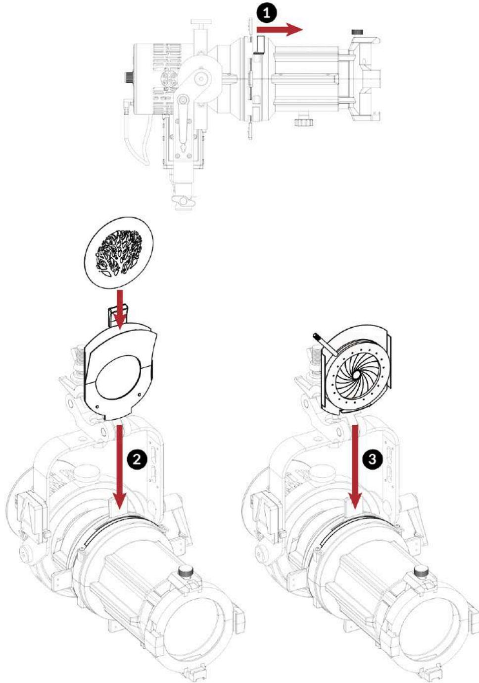
Loosen the screws on both sides of the metal slider (1) and move it aside to allow the Gobo Holder (2) or Iris (3) to slide in. Slide the metal slider (1) back into place and tighten the screws to secure the Gobo Holder (2).
